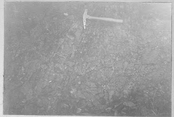
Fig. 2. Circular jointing on a horizontal surface of Bedford shale, one mile southwest of North Amherst.
