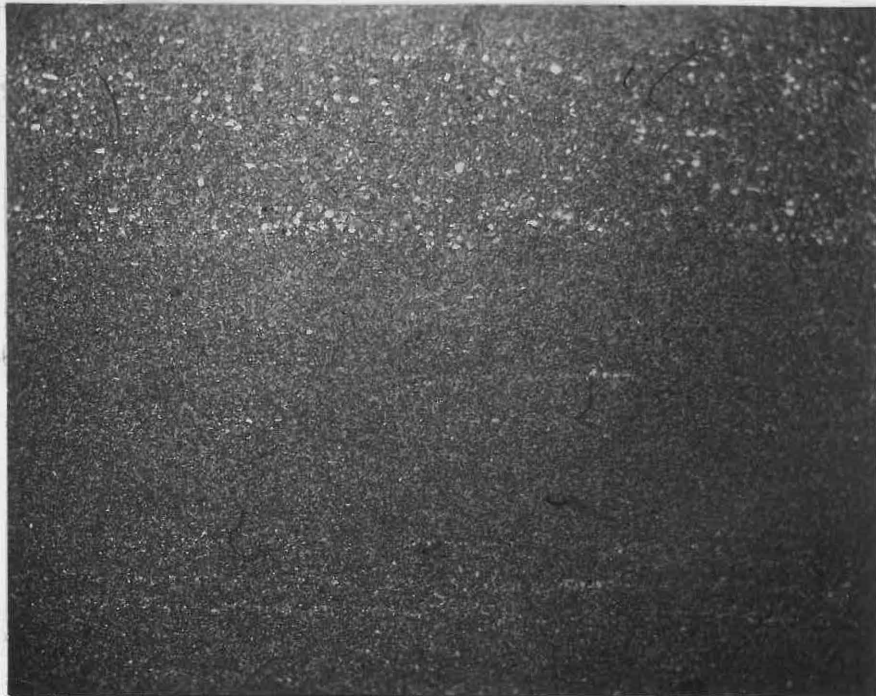
Fig.26 and Fig.27. (X-25, crossed nicols). Locality 5 - Basal layers containing much carbonate; quartz grains alined in narrow bands along plane of bedding.
