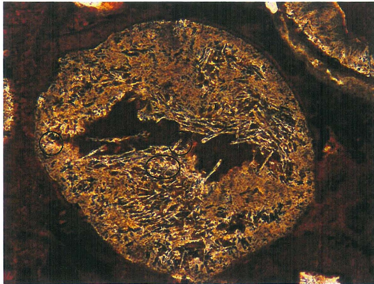
Fig. 4a- This splash form displays random to trachytic textures. The central spots are stilpnomelane while the white areas are potassium feldspar. Note the discrete crystals outlined in the stilpnomelane, this is the oval. Also within this splash form are swallow tail terminations, a crystal morphology linked with quench textures, these are circles.
