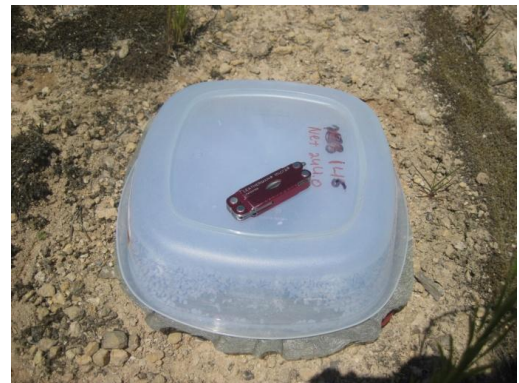
Figure 7. Photograph of container filled with desiccant used to measure water vapor mass flux at the Medicine Lake Volcano Hot Spot.
