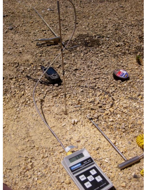
Figure 6. Photograph of equipment used to measure temperature gradients at the Medicine Lake Volcano Hot Spot.
