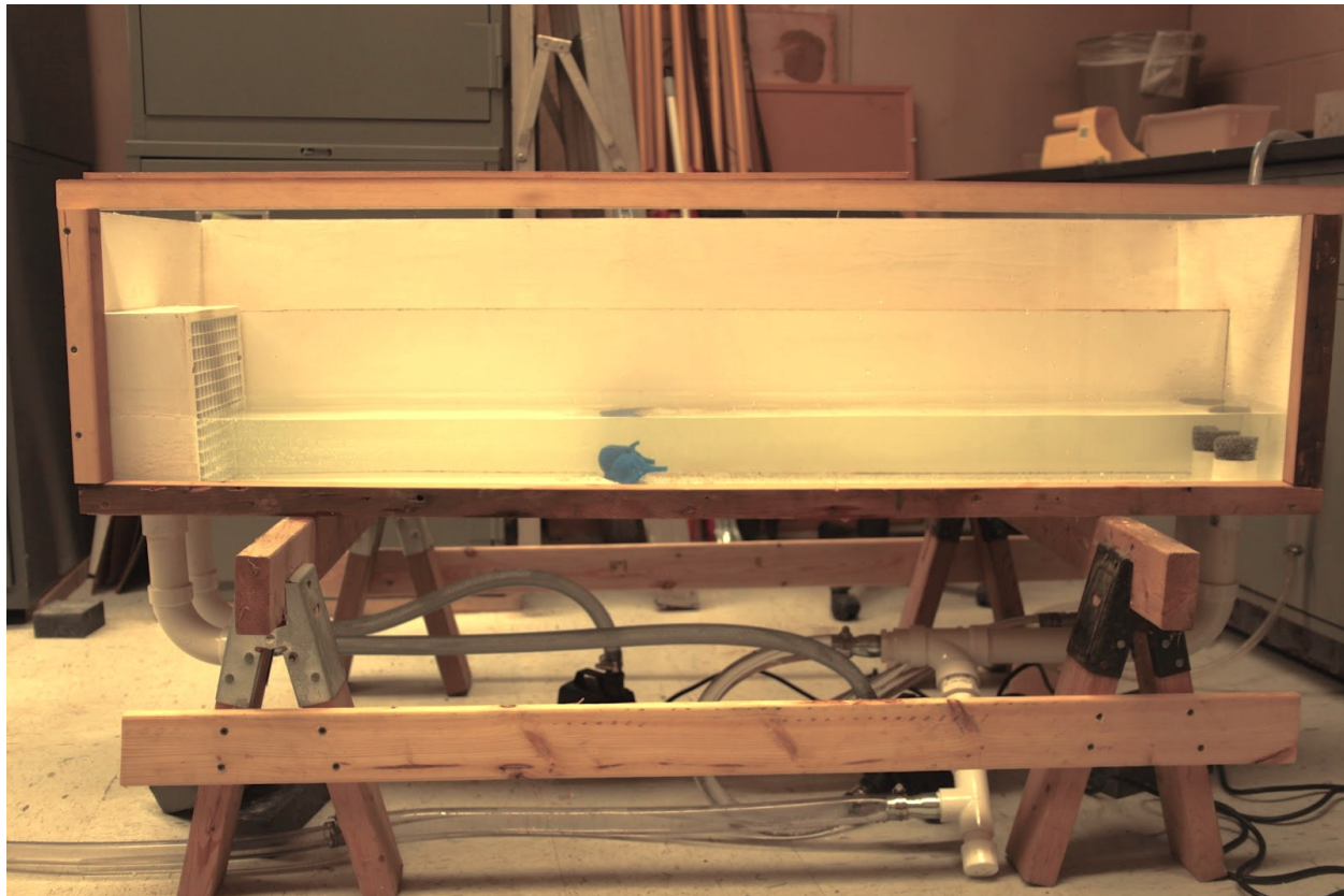
Fig IX: The HC1 hydraulic flume, specially designed for this experiment, used to assess flow around and through a model of C. tessellatus seed midway along the bed.
